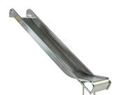
Stainless steel slide - The high quality of the materials used and solid welding guarantees high resistance to mechanical damage - 2 mm thick sheet metal, steel pipe fi 33,7 mm, durable linear welding.
