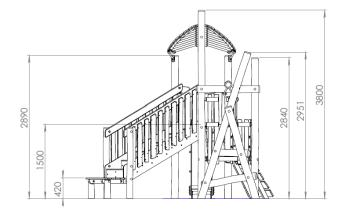
The playground equipment features a wooden structure with various play components. It includes GRP plastic slide with. With HDPE side panels which can be Substituted with a stainless steel as an option. The monkey bars works as an exercise for kids ability to climb and enter into smaller spaces improving spatial awareness and muscles. The roof reminds a leaf. Rfmt103 fature stairs that are made from HDPE panels mixed with robinia wooden material.
